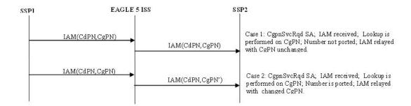
A TIF NP CgPN use case is shown in te following figure for a TIFCGPN, TIFCGPN2, or TIFCGPN3 NPP service when NPRELAY (in TIF, TIF2, or TIF3) and CGPNNP (in TIFCGPN, TIFCGPN2, or TIFCGPN3) Service Actions are provisioned and Number Portability lookup is performed on both CdPN and CgPN. A TIFCGPN, TIFCGPN2, and TIFCGPN3 NPP service is invoked by the corresponding TIF, TIF2, or TIF3 NPP Service.
