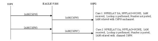
The following figure shows TIF NP Relay cases where NM bits are used in the ISUP IAM message. In the sequence diagrams, the NM bits are shown as binary values. Refer to Use of NM Bits for details on the use of NM bits.
