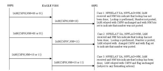
Figure 2-6 ISUP Message Flows for TIF NP Release, with Optional NM bits
