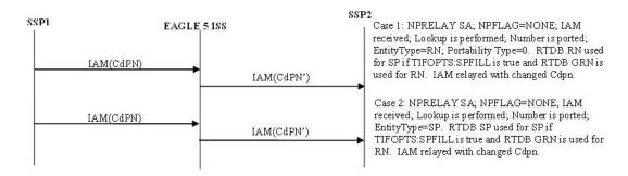
A use case using both the NPRLS and NPRELAY Service Actions is shown in the following figure. In this example, only OLO subscribers are released; own-network subscribers are relayed. The Service Actions would be set to NPRLS and NPRELAY. The NPTYPERLS configuration option is set to RN and the NPTYPERLY configuration option is set to SP.
